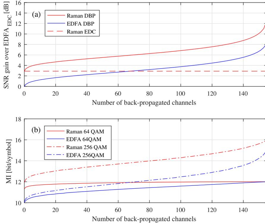
Fig. 4. (a) SNR gain over the EDFA EDC performance and (b) mutual information (MI) as a function of back-propagated bandwidth for C-band loaded Raman and EDFA amplified systems. (a) Solid lines represent the SNR after DBP, dashed line represents the EDC performance of the Raman amplified system. (b) Solid lines and dash-dot lines represent the achievable rates after DBP for EDFA and Raman systems using 64- and 256QAM respectively
