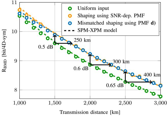
Fig. 4.  $R_{\text{BMD}}$  in bit/4D-sym vs. transmission distance in km for the SPM-XPM model of Sec. III (dashed lines) with 64QAM input and SSFM simulations (markers). The colors represent the different PMFs: uniform input (green), SNR-dependent shaped PMFs (orange), and the SNR-independent PMF **d)** of Table I (blue).
