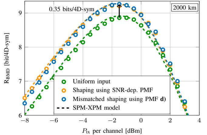
Fig. 5.  $R_{\text{BMD}}$  in bit/4D-sym vs.  $P_{\text{tx}}$  per channel in dBm for 64QAM. The SPM-XPM model results (dashed lines) for uniform input, SNR-dependent shaping and shaping with a fixed PMF are shown. For the latter, the distribution **d)** of Table I is used for all launch powers. SSFM simulation results (markers) validate the SPM-XPM model.
