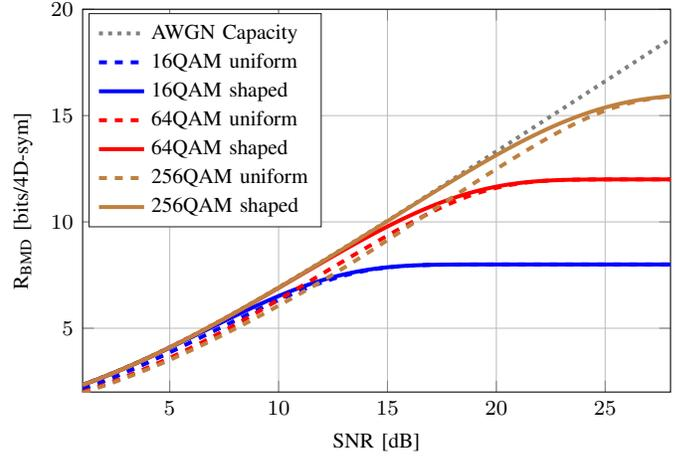
Fig. 2.  $R_{\text{BMD}}$  in bits/4D-sym for uniform QAM input (dashed lines) and QAM with the shaped, SNR-dependent MB PMF of (14) (solid lines). The AWGN capacity (dotted line) is shown as a reference.
