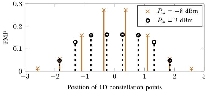
Fig. 8. Optimized 1D PAM PMFs for  $P_{\text{tx}} = -8$  dBm (solid, crosses) and  $P_{\text{tx}} = 3$  dBm (dashed, circles). Although these two power levels have approximately the same  $\text{SNR}_{\text{eff}}$ , the PMF for 3 dBm is less shaped to avoid increased NLI.
