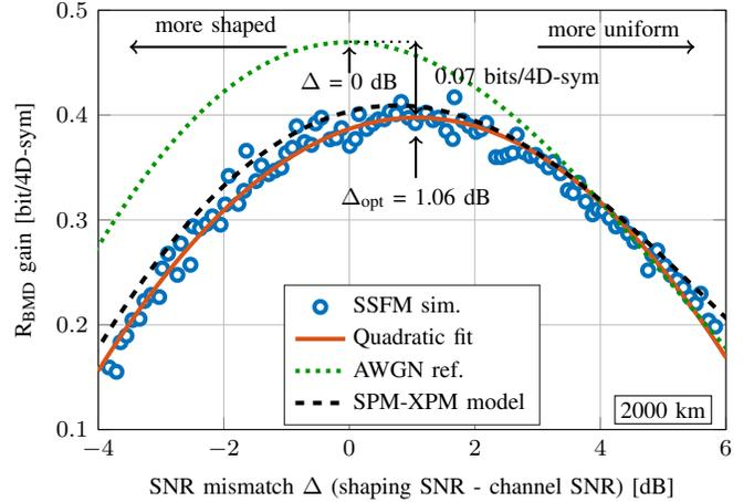
Fig. 7.  $R_{\text{BMD}}$  gain in bit/4D-sym of shaped 64QAM over uniform 64QAM vs. SNR mismatch  $\Delta$  in dB. The solid line is a quadratic fit to the simulations and has its maximum at  $\Delta_{\text{opt}} = 1.06$  dB. The SPM-XPM model (dashed line) correctly predicts the trend of the simulations. The dotted line shows as a reference the BMD rate gain for an AWGN channel with 14.17 dB SNR where the maximum shaping gain is obtained in the case of no SNR mismatch, i.e.,  $\Delta = 0$  dB.
