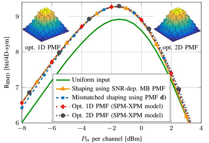
Fig. 9.  $R_{\text{BMD}}$  in bit/4D-sym for 64QAM vs.  $P_{\text{tx}}$  per channel in dBm for the SPM-XPM model. The AIRs for the 1D-optimized input (red dotted), for the 2D-optimized PMF (gray dotted) and for all other shaped inputs lie on top of each other over a wide range of launch powers. Inset: The optimized 1D PMF in its 2D representation and the 2D PMF, each for  $P_{\text{tx}}$  of -1.5 dBm.
