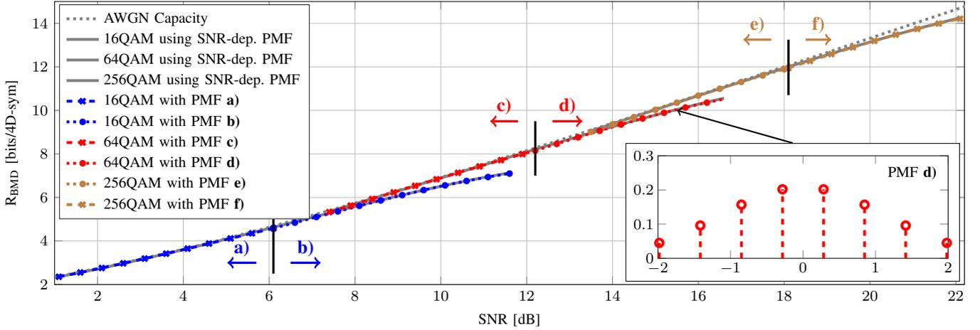
Fig. 3.  $R_{\text{BMD}}$  in bits/4D-sym for 16QAM, 64QAM, and 256QAM over the AWGN channel. The QAM formats shaped with SNR-dependent PMFs are shown as reference (gray solid lines), and shaping with fixed PMFs a) to f) is shown as colored lines with markers, with the respective SNR intervals indicated by vertical black lines. The inset shows the mismatched PMF d) that is used for SNRs from 12.2 dB to 16.6 dB. Details on the fixed distributions are given in Table I.
