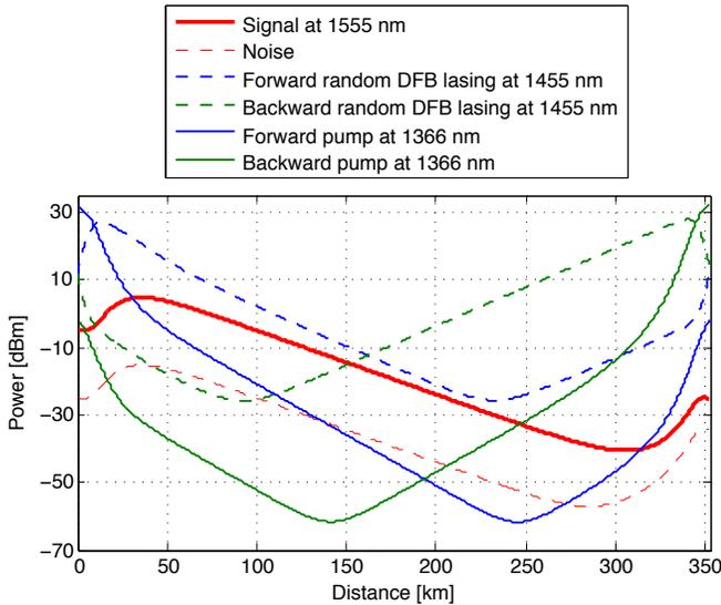
Fig. 5. Simulation of signal (solid red), noise -measured in 0.1 nm bandwidth (dashed red), forward pump (solid blue), backward pump (solid green), forward lasing (dashed blue) and backward lasing (dashed green) power evolution in the 352.8 km link.
