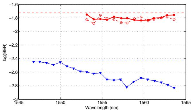
Fig. 8. Experimental BER results in 327.6 km (triangle) and experimental (solid) and simulated (dashed) in 352.8 km (circle) link. Horizontal dashed lines indicates hard- ( $3.8 \times 10^{-3}$ ) and soft- ( $1.9 \times 10^{-2}$ ) decision FEC limit.
